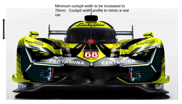
Minimum cabin height to be increased to 55mm Furthest point forward must be above axle line. (Axle line set 15mm above reference plane)
