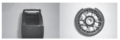
Wheels must use a 17mm hex hub consistent with the dimensions and function of the hubs used in 1/8 off road racing. The wheel must be affixed by a 17mm wheel nut, threaded on to the hex hub. Quick change mechanisms are not permitted.
